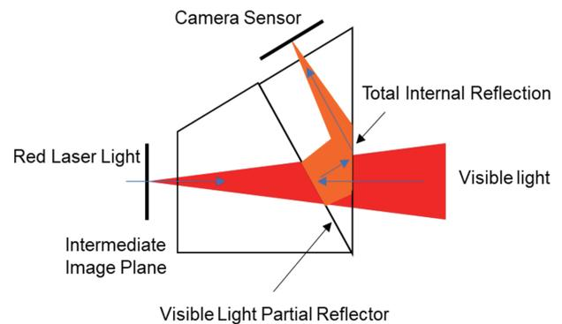
Fig. 6 Dichroic prism.
